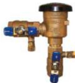
**A pressure vacuum breaker like the one shown here is the most common type of residential backflow prevention device. However, some systems may be equipped with a reduced pressure principle backflow preventer or atmospheric vacuum breakers located downstream of control valves.**
